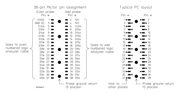
Five center inline pins on the connector are the signal ground returns and must be connected to ground.
