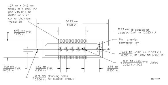
The high-density connector pin assignment and recommended circuit board routing are shown in the following figure.
